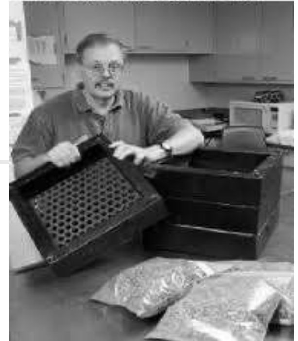
Figure 1. The Penn State particle size separator can be used to monitor silage particle size.
